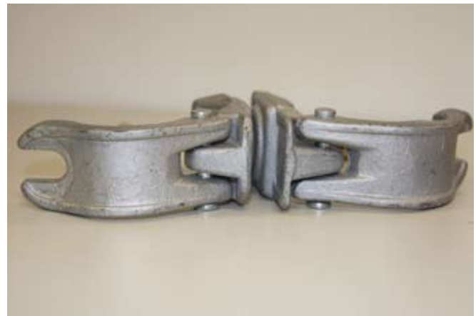
Example of unmarked scaffold coupler
