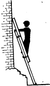
Figure 19 Correct arrangement of ladder. Base about 1 out from wall to 4 vertical height. Horizontal benching of ground ensures vertical alignment of ladder.
